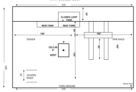
Strong back: 30' towards the pipe rack end 60'x40' 30' towards the power end 20' on each side of the well
