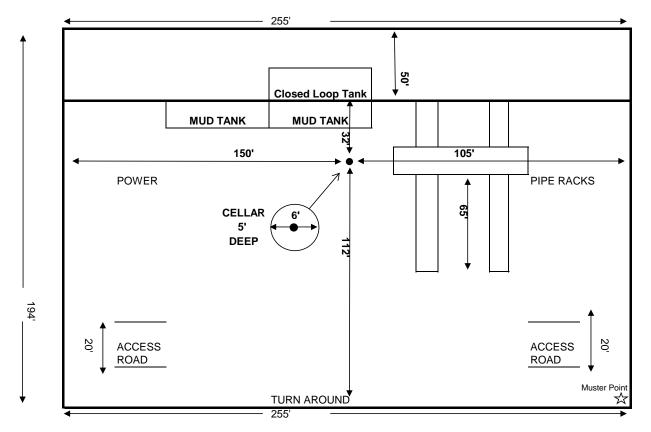
RIG 1 - RAT HOLE 9'2" OUT TO TURN AROUND SIDE. 7'10" TO PIPE RACKS, MOUSE HOLE 3' 3" TO PIPE R
